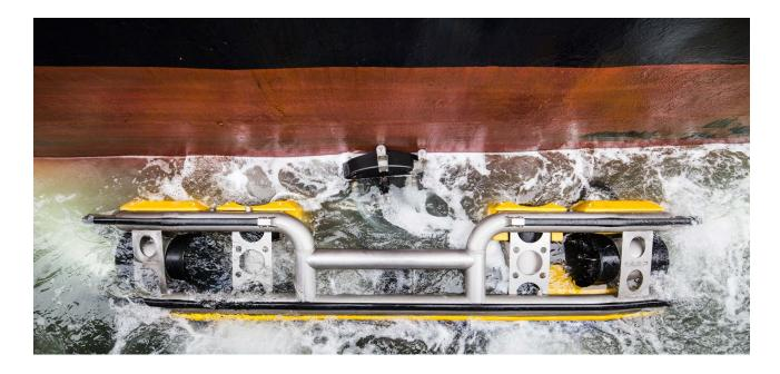
The HullWiper Remotely Operated Vehicle (ROV) is a diver- and brush-free system that can clean whilst operations like loading/discharging of bunker deliveries are underway, saving you valuable time and money. Cleaning with HullWiper's ROV can be carried out in most weather conditions.
